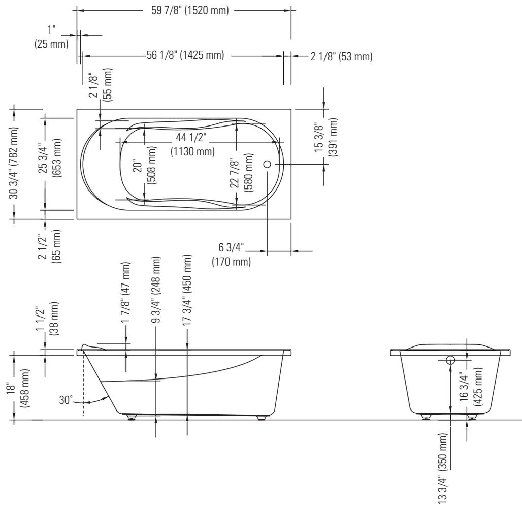
\*A bathtub fitted with back jets can cause the pump to protrude by approximately 3" from the overall dimension.
